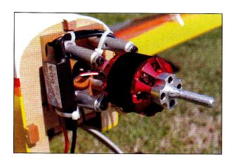
Always make sure the components you use have a good amount of headroom. Some use a figure of 20%. gives us the maximum power, whilst simultaneously keeping the current at a level within the limits of both the ESC and the motor.
